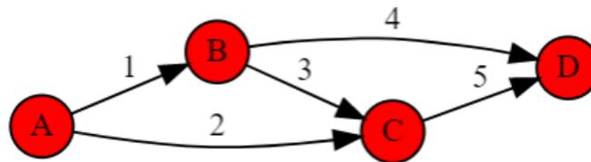
A, B, C, and D are **nodes**. The nodes are connected by **arcs**, labeled 1 through 5. In this example, there are several paths from A to D, but all must pass through either B or C (or both). If the network flows model is compared to a road map, the nodes are intersections and the arcs are the roads that can be taken at that intersection.
